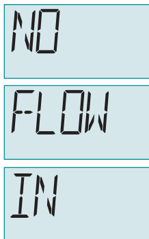
Figure 3-4 NO FLOW IN Alarm
