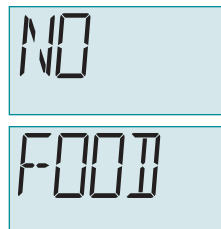
Figure 3-6 NO FOOD Alarm
