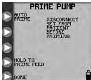
Figure 8A. PRIME PUMP menu for feed-only set.
