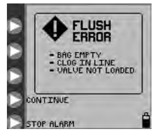
Figure 28. Flush Error screen.
