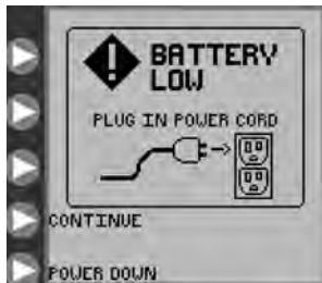
Figure 31. Battery Low error screen. Indicates that the battery must be recharged immediately.
